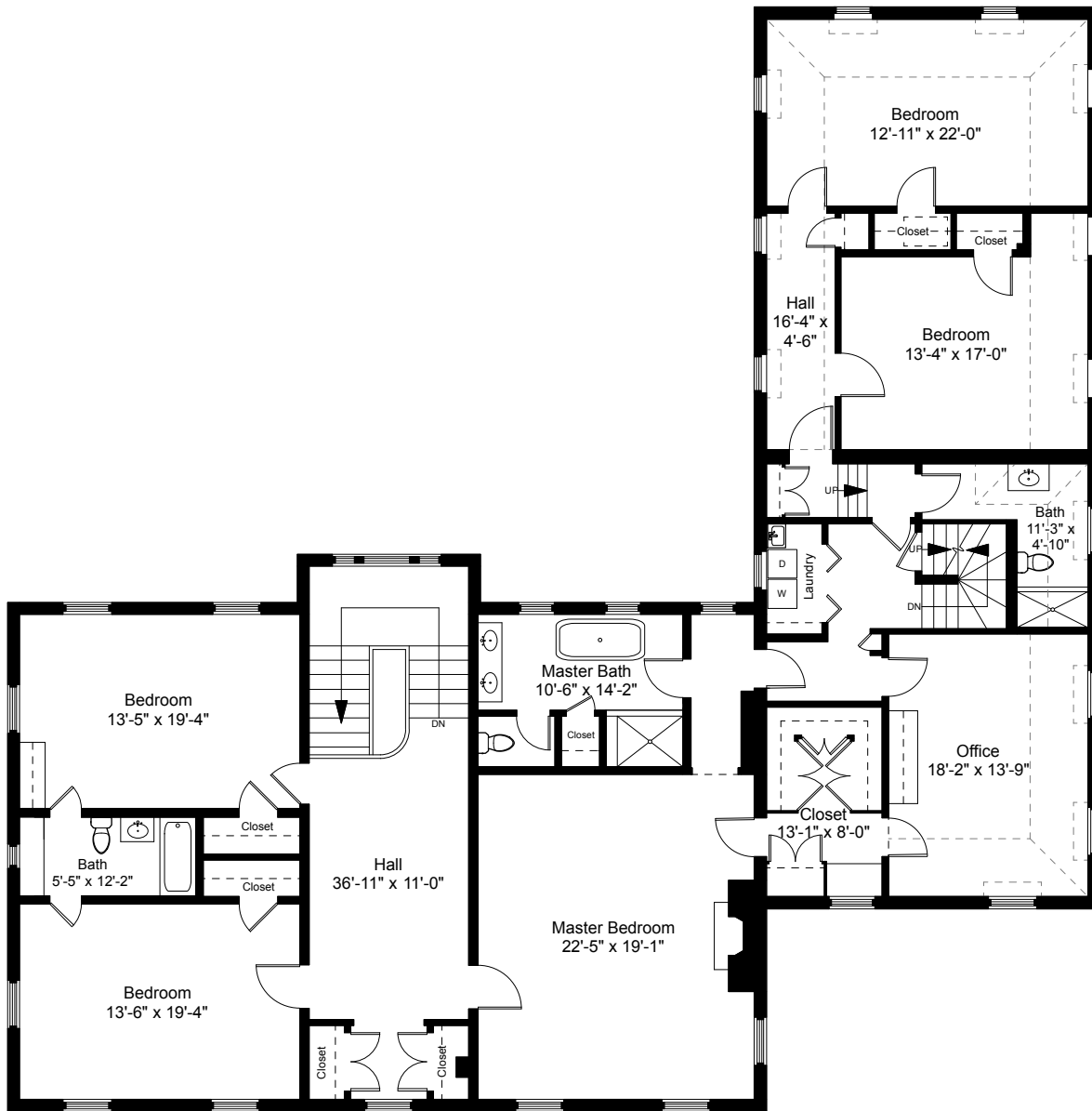
Second Floor Plan Ceiling Height = 9'-6"
